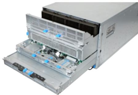
The architecture is designed around a toolless modular philosophy. Major components can be removed from the system chassis without unmounting from the rack for better serviceability and increased system uptime. The modularity in this innovative design allows for forward support of next generation CPUs and GPUs.
